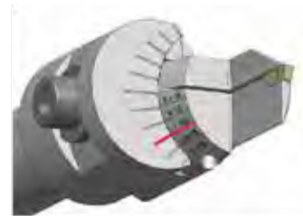
Mark = 7 1/4 setting, D min = 5" D max = 9.5"
