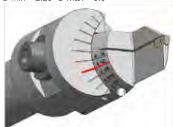
Mark = 9 1/2 setting, D min = 8" D max = 11"
