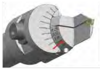
Mark = 4 9/16 setting, D min = 3.375" D max = 5.75"
