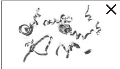
Apple-peel-like chips (Without curling)
