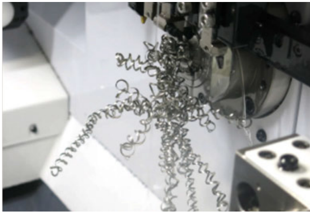
External coolant supply at normal pressure
