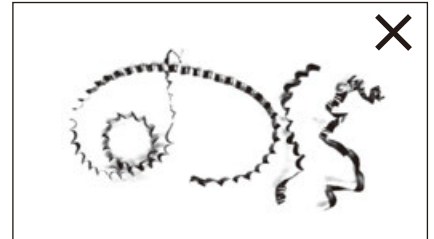
Continuously coiled long chips
