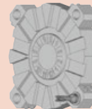
Scale for adjusting cutting edge height in turning (Front face of sleeve)
