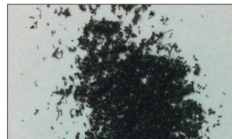
Chips are nearly like dust. Pressurized air coolant recommended to blow away chips.
